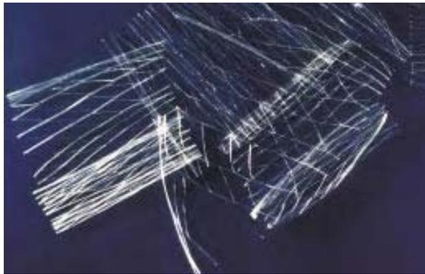
These bundles of fibrillated polypropylene fibers open up as the concrete is mixed, forming a more tenacious bond with the cement paste than monofilament fibers.
